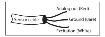
The red wire connects to the positive supply and the white wire to the negative supply. The shield (bare
